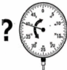
Reading errors: • \pm sign error • parallax error • mirror image readings
